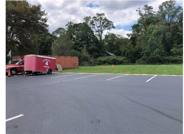
Parking spaces can be converted to porous pavement to capture and infiltrate stormwater runoff from the parking lot. A rain garden can be installed in the turfgrass area near the entrance of the building to capture, treat, and infiltrate stormwater runoff from the roof. A preliminary soil assessment suggests that more soil testing would be required before determining the soil's suitability for green infrastructure.
