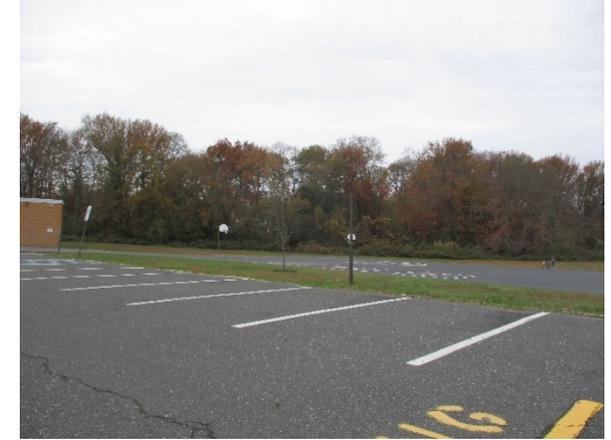
Parking spaces can be converted to porous pavement to capture and infiltrate stormwater runoff from the parking lot. Rain gardens can be installed in the turfgrass areas around the school to capture, treat, and infiltrate stormwater runoff from the roof. A preliminary soil assessment suggests that more soil testing would be required before determining the soil's suitability for green infrastructure.
